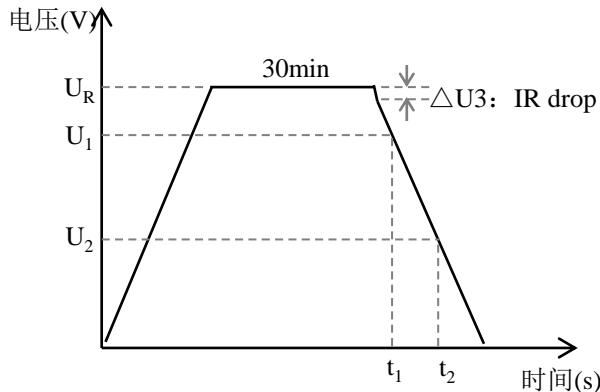
$$\text{容量计算公式: } C = \frac{I \times (t_2 - t_1)}{U_1 - U_2}$$
