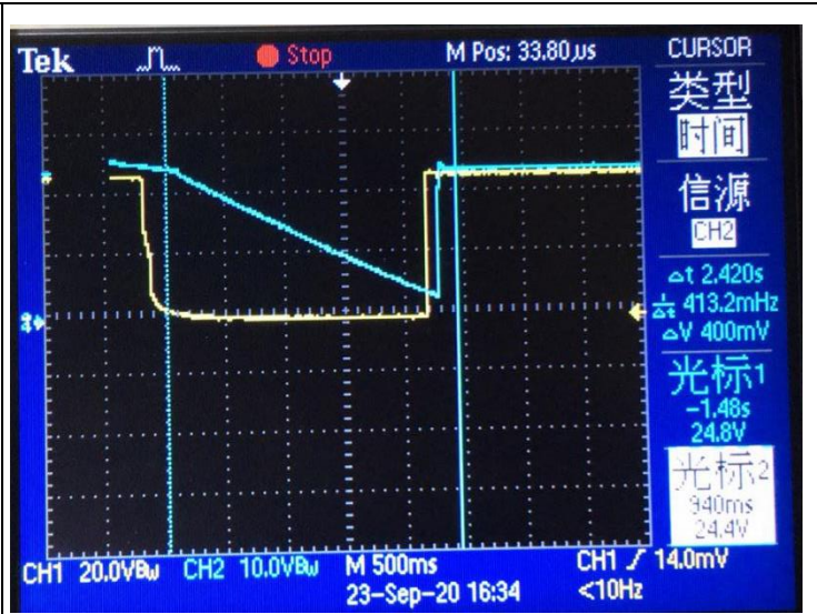
Output response & load (24V / 0.01A)
