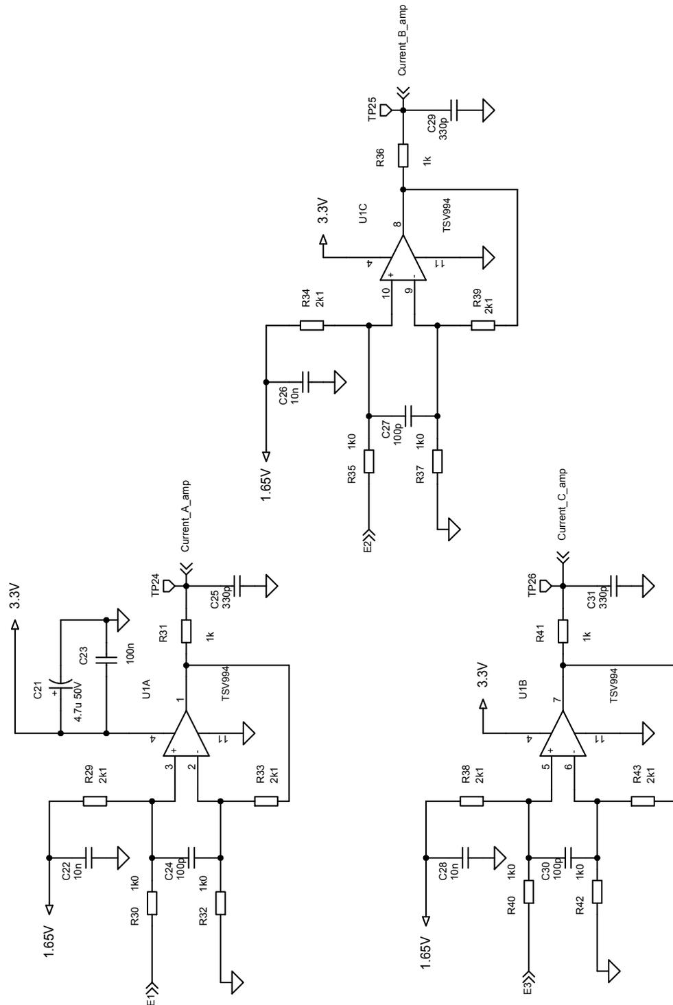
Figure 6. STEVAL-IPM10B circuit schematic (6 of 6)
