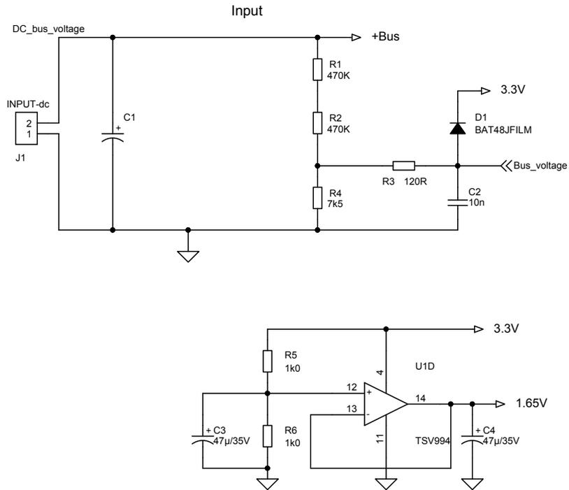
Figure 4. STEVAL-IPM10B circuit schematic (4 of 6)
