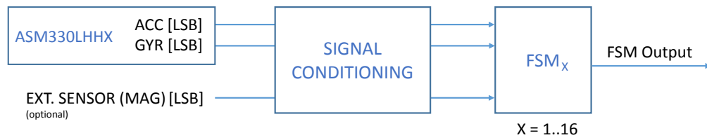
Figure 2. State machine in the ASM330LHHX
