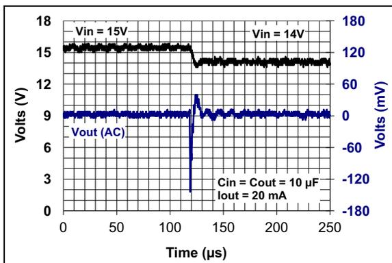
**FIGURE 2-9:** 12V LDO Dynamic Linestep - Falling  $V_{DD}$ .
