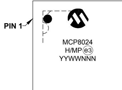
48-Lead TQFP (7x7)
