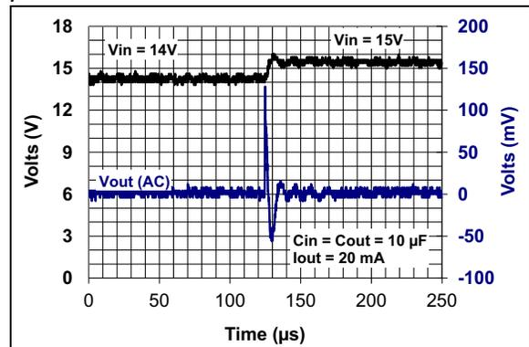
**FIGURE 2-6:** 5V LDO Dynamic Linestep - Rising  $V_{DD}$ .
