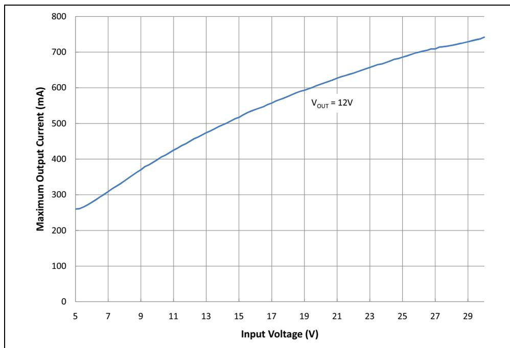
**FIGURE 2-1:** Typical Maximum Output Current vs. Input Voltage
