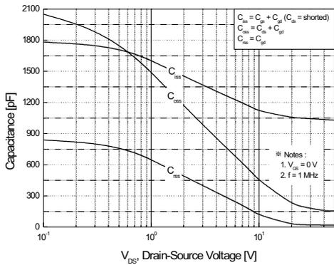
Figure 5. Capacitance Characteristics
