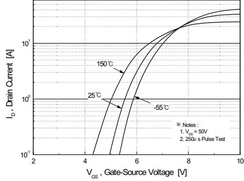
Figure 2. Transfer Characteristics
