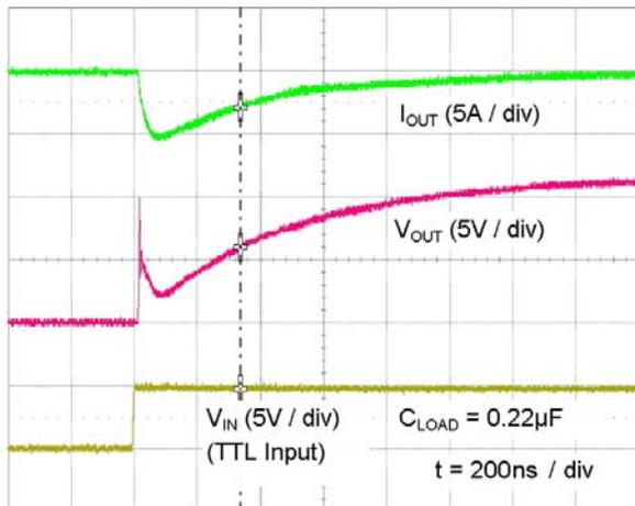
Figure 42. Quasi-Static Source Current with  $V_{DD}=12\text{ V}^{(16)}$
