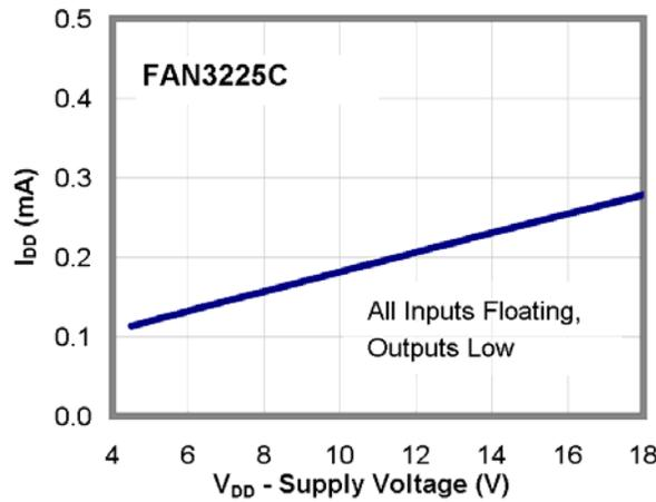
Figure 14.  $I_{DD}$  (Static) vs. Supply Voltage<sup>(15)</sup>
