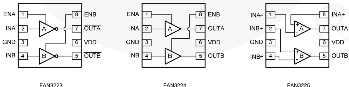
Figure 1. Pin Configurations
