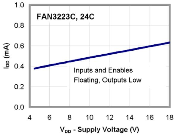
Figure 12.  $I_{DD}$  (Static) vs. Supply Voltage<sup>(15)</sup>
