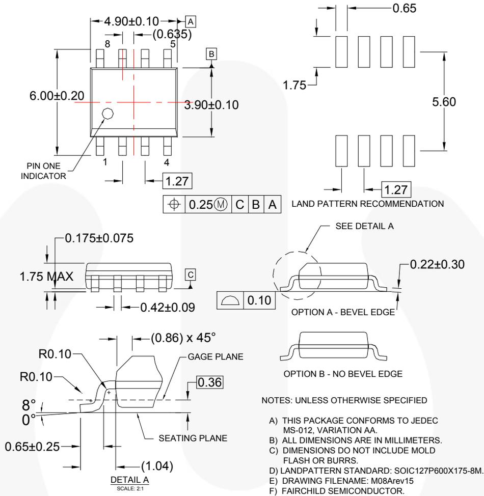
Figure 58. 8-Lead Small Outline Integrated Circuit (SOIC)
