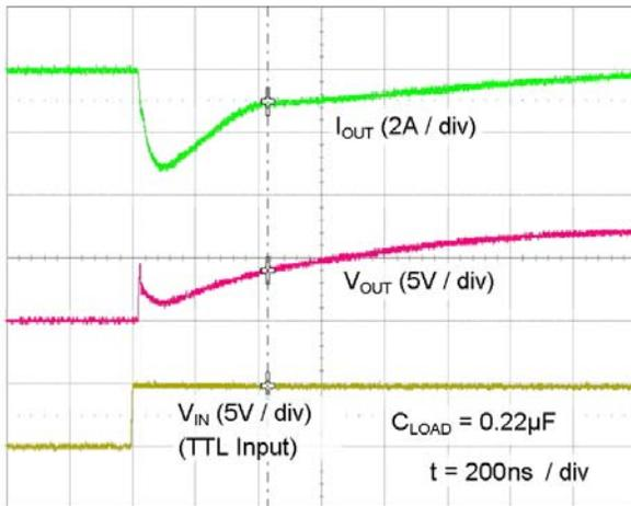
**Figure 44. Quasi-Static Source Current with  $V_{DD}=8\text{ V}$ <sup>(16)</sup>**
