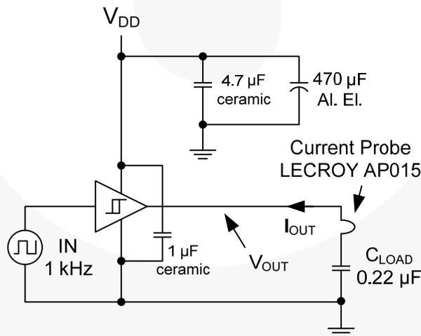
**Figure 46. Quasi-Static  $I_{OUT}$  /  $V_{OUT}$  Test Circuit**
