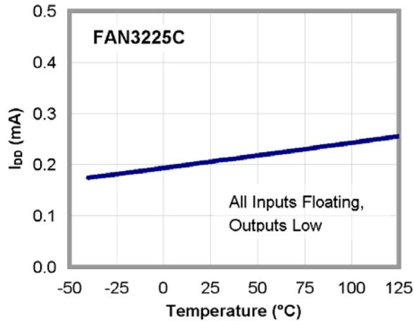
Figure 21.  $I_{DD}$  (Static) vs. Temperature<sup>(15)</sup>
