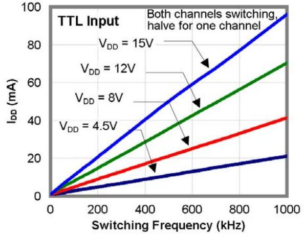
Figure 18.  $I_{DD}$  (2.2 nF Load) vs. Frequency
