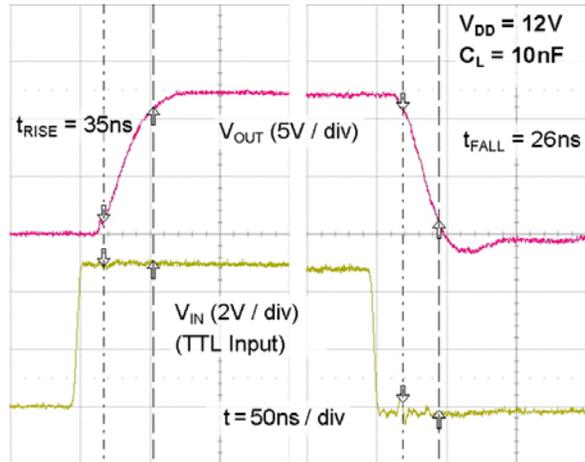
Figure 41. Rise/Fall Waveforms with 10 nF Load
