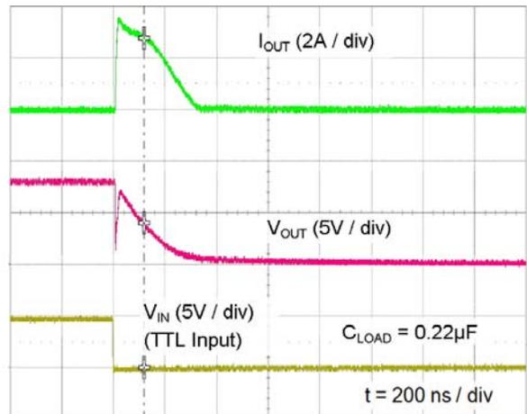
Figure 43. Quasi-Static Sink Current with  $V_{DD}=12\text{ V}^{(16)}$
