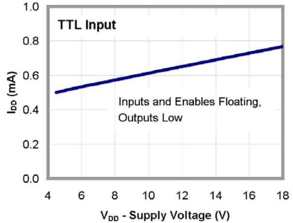
Figure 13.  $I_{DD}$  (Static) vs. Supply Voltage<sup>(15)</sup>
