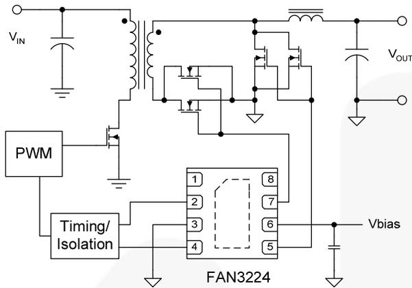
**Figure 54. High Current Forward Converter with Synchronous Rectification**
