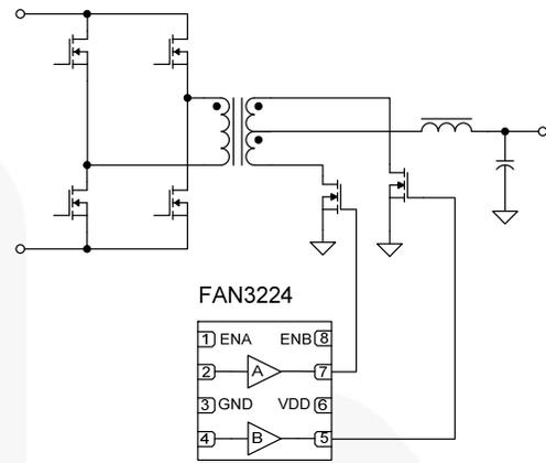
**Figure 55. Center-Tapped Bridge Output with Synchronous Rectifiers**
