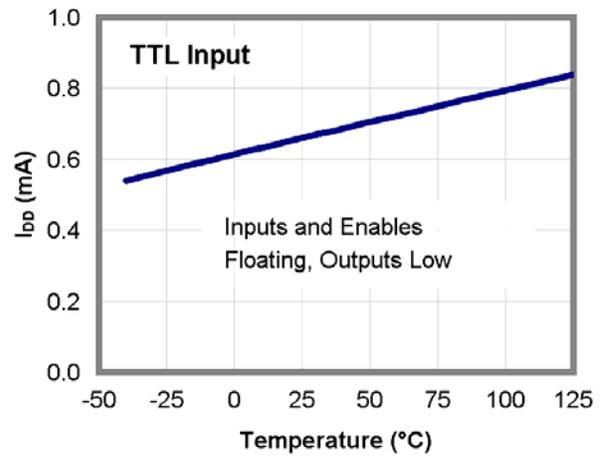
Figure 20.  $I_{DD}$  (Static) vs. Temperature<sup>(15)</sup>
