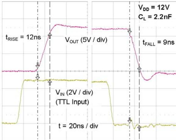
Figure 40. Rise/Fall Waveforms with 2.2 nF Load
