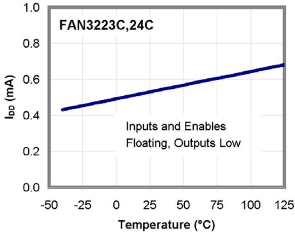
Figure 19.  $I_{DD}$  (Static) vs. Temperature<sup>(15)</sup>
