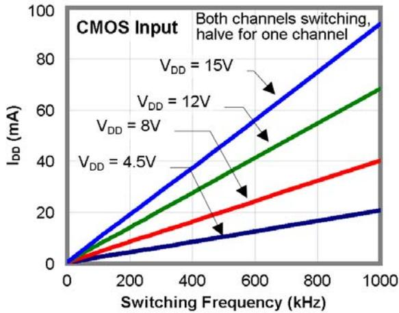
Figure 17.  $I_{DD}$  (2.2 nF Load) vs. Frequency
