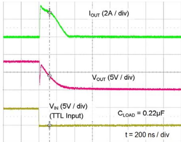
**Figure 45. Quasi-Static Sink Current with  $V_{DD}=8\text{ V}$ <sup>(16)</sup>**
