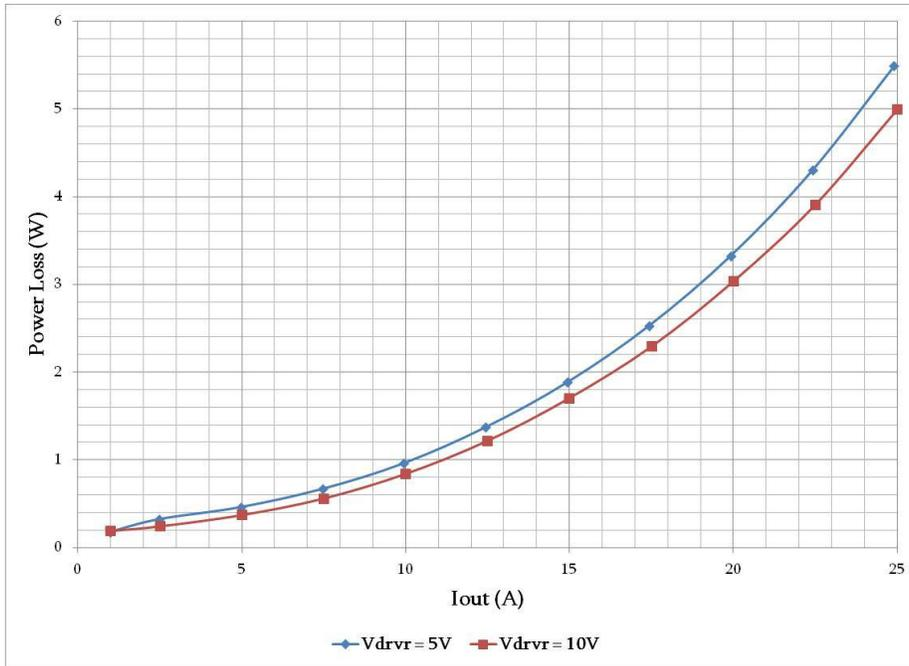
Figure 7: Comparison of Power Loss for ONS321G Board for  $V_{drvr} = 5V$  &  $10V$
