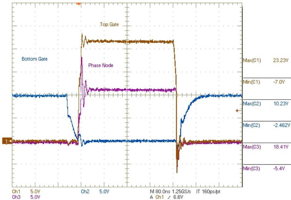
Figure 9: Switch Node Waveforms for  $V_{drv} = 10V$
