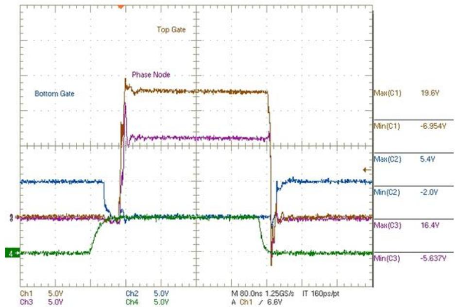
Figure 11: PWM signal at G1 for  $I_{out} = 20A$
