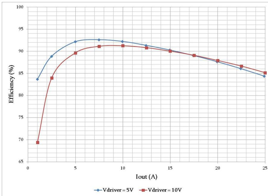
Figure 5: Comparison of Efficiency for ONS321G Board for V<sub>drv</sub> = 5V & 10V
