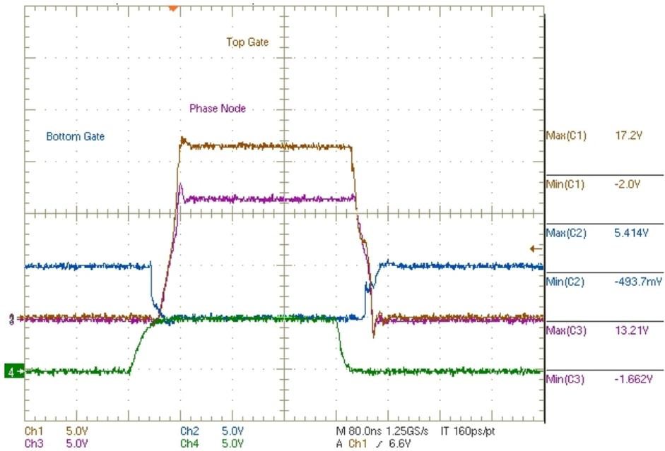
Figure 10: PWM Signal at G1 for  $I_{out} = 0A$
