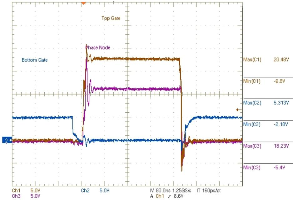
Figure 8: Switch Node Waveforms for  $V_{drv} = 5V$
