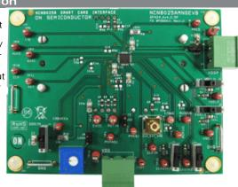
the industry standard features usually required for STB smart card interface. It is also offered in a very compact package profile, QFN-16 (NCN8025), satisfying the requirements of cost efficiency and space saving requested by CAM and SIM applications. For details regarding device implementation refer to the application note AND8003 available under request (please contact local sales office or representative).
