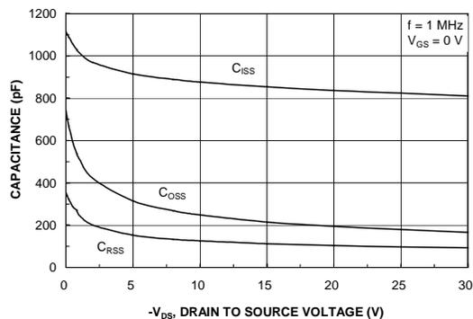
Figure 8. Capacitance Characteristics.
