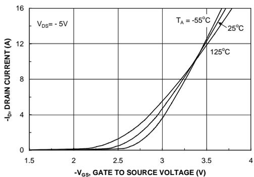
Figure 5. Transfer Characteristics.
