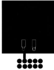
a) 40 °C/W when mounted on a 1 in<sup>2</sup> pad of 2 oz copper
