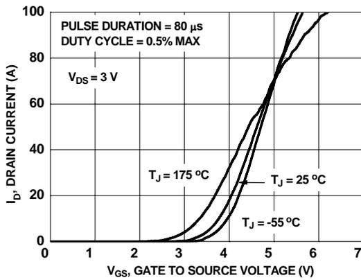
**Figure 5. Transfer Characteristics**
