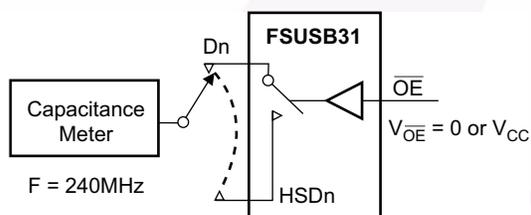
**Figure 20. Channel Off Capacitance**
