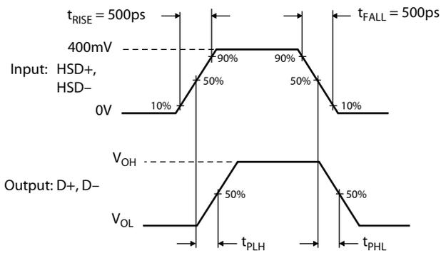
**Figure 12. Switch Propagation Delay Waveforms ( $t_{PD}$ )**
