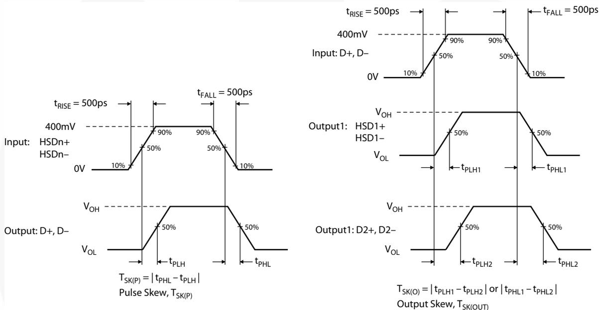
**Figure 15. Switch Skew Tests**
