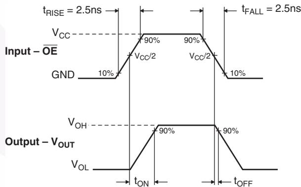
**Figure 13. Turn On / Turn Off Waveform ( $t_{ON} / t_{OFF}$ )**
