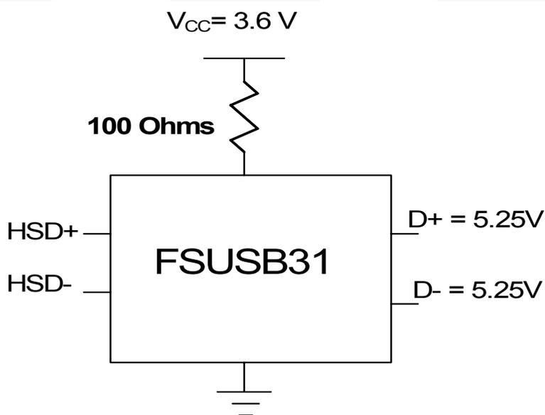
**Figure 21. A 100Ω resistor in series with the V<sub>CC</sub> supply allows the FSUSB31 to withstand a Vbus short when powered up**
