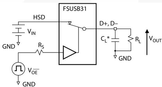
$R_L$ ,  $R_S$ , and  $C_L$  are functions of the application environment (see AC Electrical tables for specific values).
