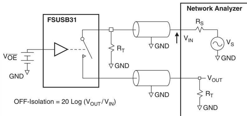
**Figure 17. Channel Off Isolation**
