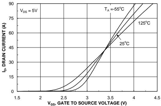
Figure 5. Transfer Characteristics
