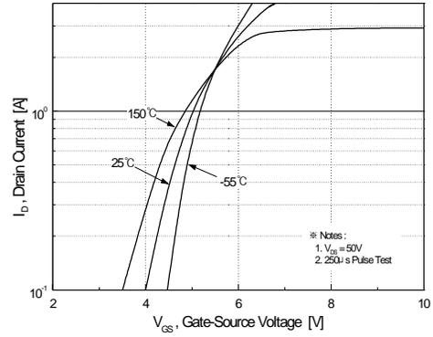
Figure 2. Transfer Characteristics
