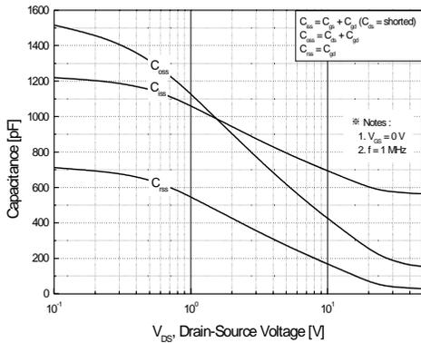
Figure 5. Capacitance Characteristics
