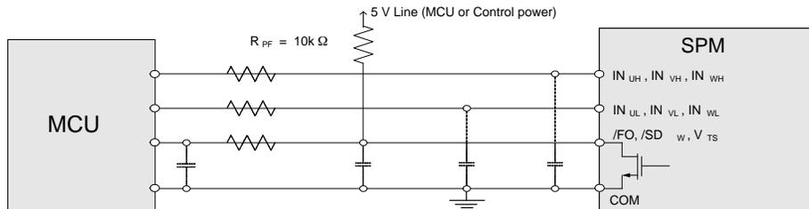
NOTE: RC coupling at each input (parts shown dotted) might change depending on the PWM control scheme used in the application and the wiring impedance of the application's printed circuit board. The input signal section of the SPM 8 product integrates 5 kΩ (typ.) pull-down resistor. Therefore, when using an external filtering resistor, please pay attention to the signal voltage drop at input terminal.
