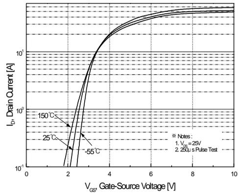
**Figure 2. Transfer Characteristics**
