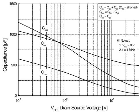
**Figure 5. Capacitance Characteristics**
