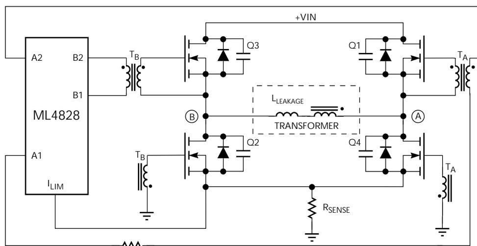
Figure 1. Simplified diagram of Phase Modulated power Outputs.
