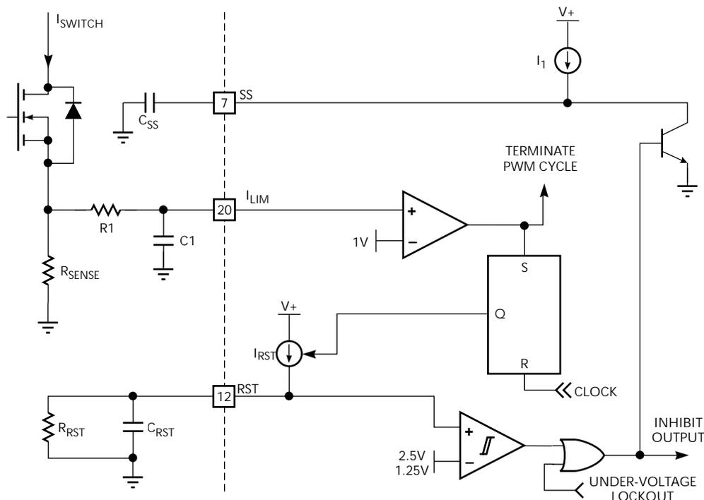
Figure 5. Over-Current, Soft-Start, and Integrating Fault Detect Circuits.
