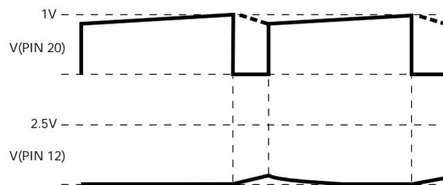
Figure 6.  $I_{LIM}$  and Resulting  $RC_{RST}$  Waveforms During Load Surge.
