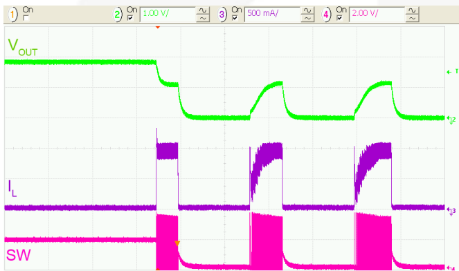
Figure 35. Over-Current Fault Response, R_{LOAD} = 1\ \Omega , 50\ \mu\text{s}/\text{div} .
