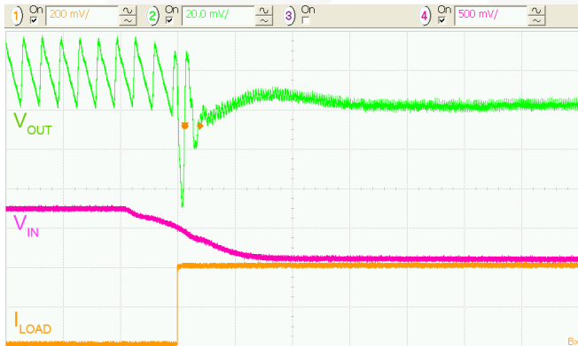
Figure 22. Combined Line/Load Transient 3.9 to 3.3 V_{IN} Combined with 40 mA to 400 mA Load Transient
