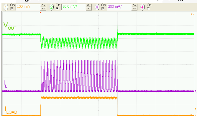
Figure 30. Load Transient 0 to 150 mA, 4.5 V_{IN}
