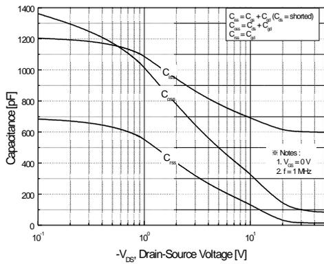
Figure 5. Capacitance Characteristics
