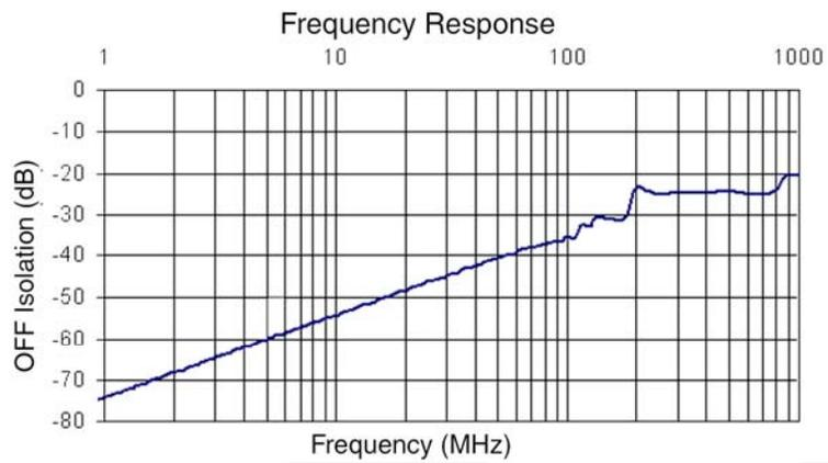
**Figure 5. Off Isolation ( $V_{BAIS}=0.5V$ ,  $V_{CC}=3.0V$ ,  $SEL_n=LOW$ )**
