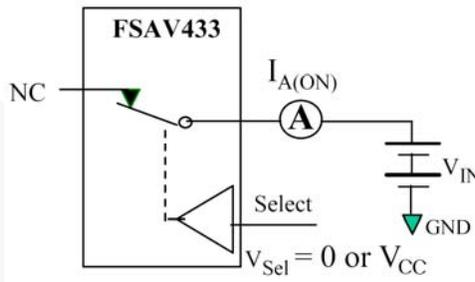
**Figure 11. On Leakage**
