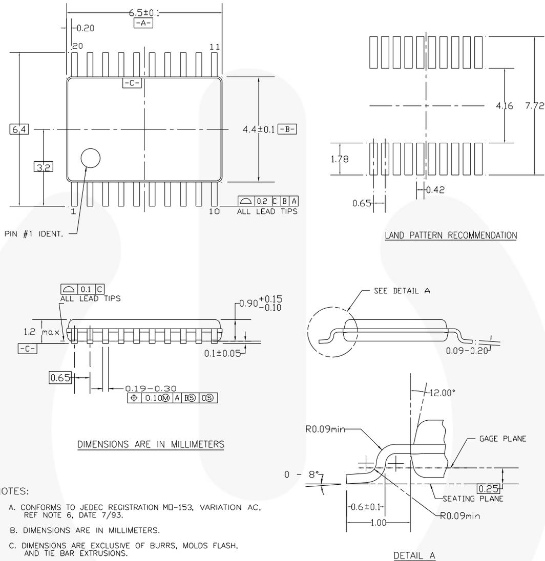
**Figure 18. 20-Lead, Thin Shrink Small Outline Package (TSSOP)**
