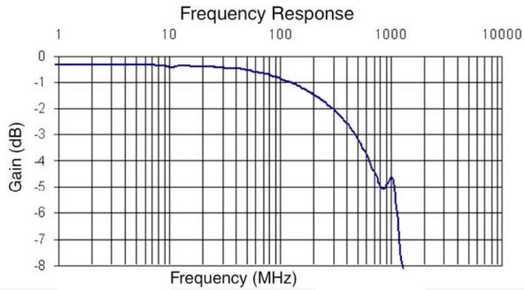
**Figure 4. Gain vs. Frequency ( $V_{BAIS}=0.5V$ ,  $V_{CC}=3.6V$ ,  $R_L=50\Omega$ )**
