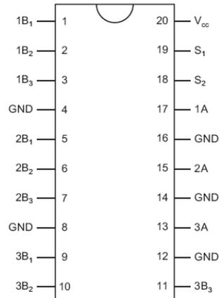
Figure 3. TSSOP Pin Assignments (Top Through View)
