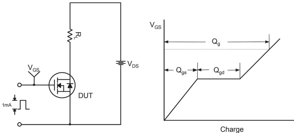
**Figure 14. Resistive Switching Test Circuit & Waveforms**
