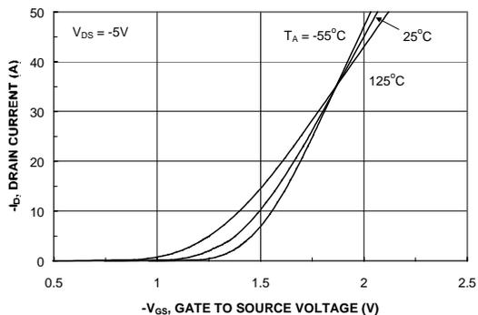
Figure 5. Transfer Characteristics.
