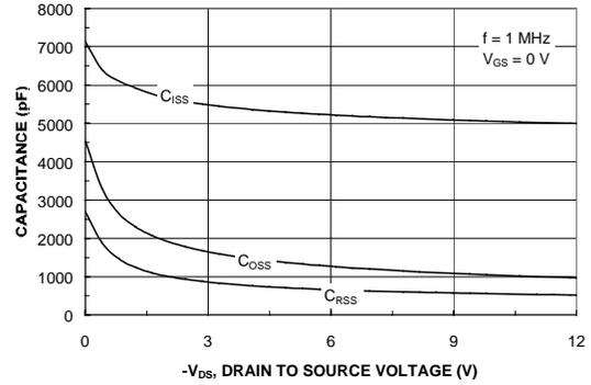
Figure 8. Capacitance Characteristics.
