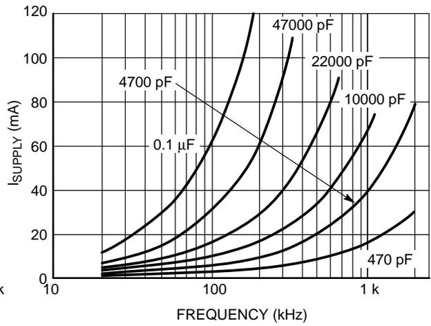
Figure 13. Supply Current vs. Frequency ( $V_{DD} = 6\text{ V}$ )
