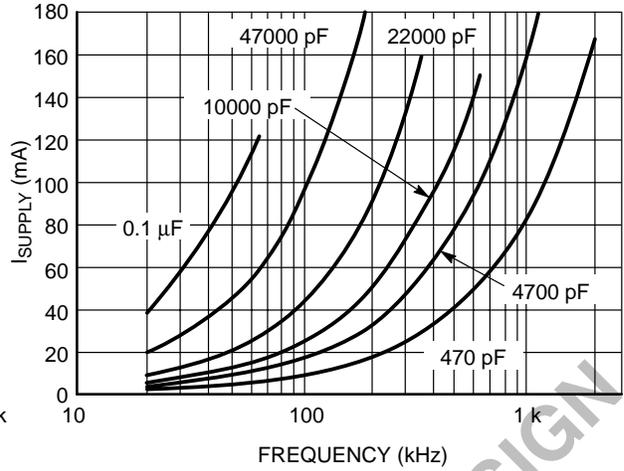
Figure 9. Supply Current vs. Frequency ( $V_{DD} = 18\text{ V}$ )
