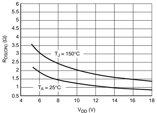
Figure 19. Low-State Output Resistance vs. Supply Voltage
