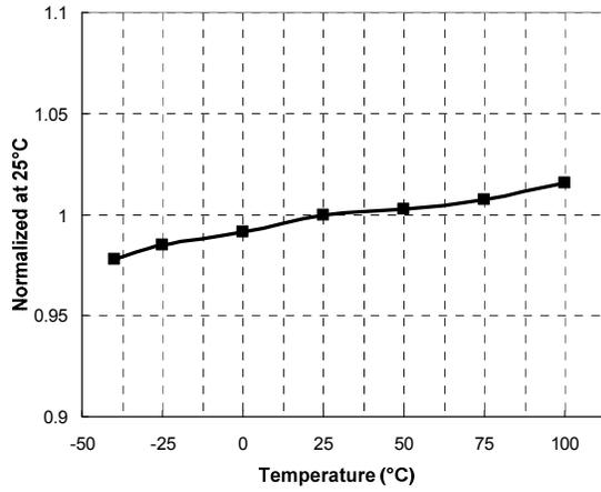
**Figure 4. Low-Side MOSFET Duty Cycle vs. Temperature**
