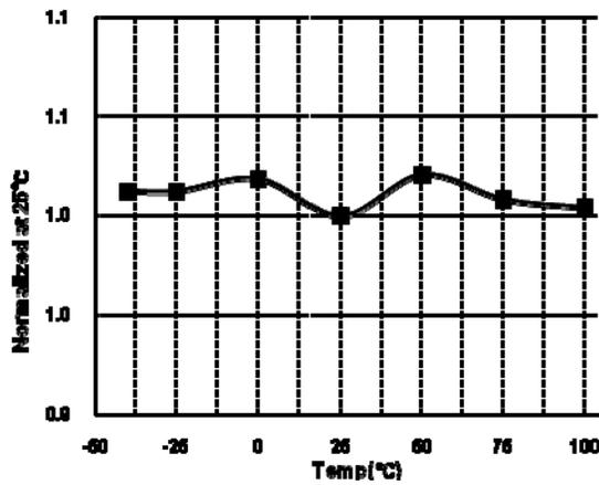
Figure 12. V<sub>RT,RESET</sub> vs. Temperature
