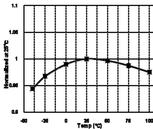
Figure 15. I<sub>LINE</sub> vs. Temperature
