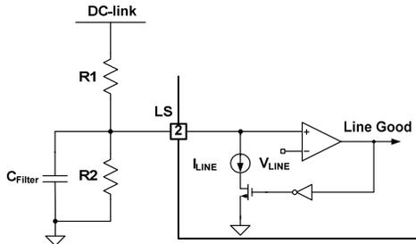
Figure 25. Half-Wave Sensing
