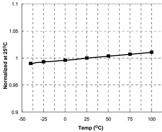
Figure 10. LV<sub>CC</sub> OVP Voltage vs. Temperature
