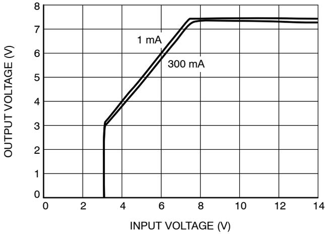
**Figure 3. Dropout Characteristics**
