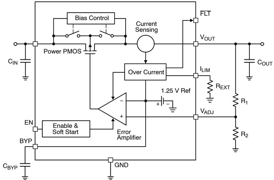
Figure 2. CAT6201/CAV6201B Functional Block Diagram
