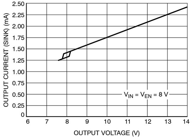
Figure 14. Output Current (Sink) vs. Output Voltage
