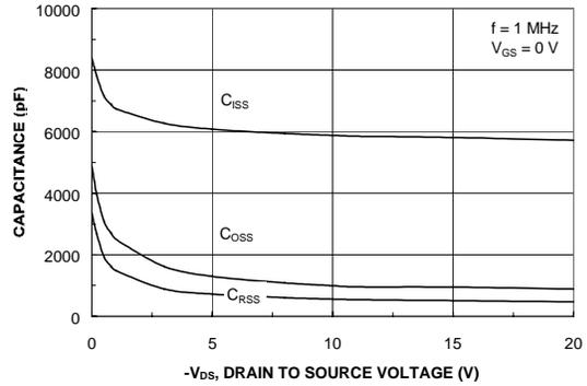
Figure 8. Capacitance Characteristics.
