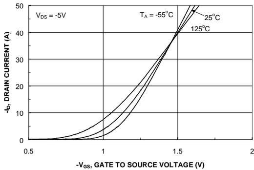
Figure 5. Transfer Characteristics.
