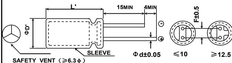
When  $\Phi D \leq 8$ ,  $\Phi D' \leq \Phi D + 0.5$ , and  $L' \leq L + 1.5$
