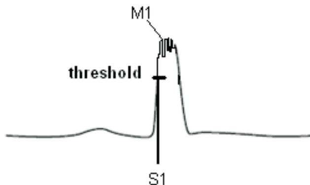
6. After detecting a QRS peak, the next 50 samples (SKIP\_WINDOW = 50) are skipped to take care of the minimum RR interval that can occur in the case of maximum detectable heart rate (i.e. 240 BPM).
