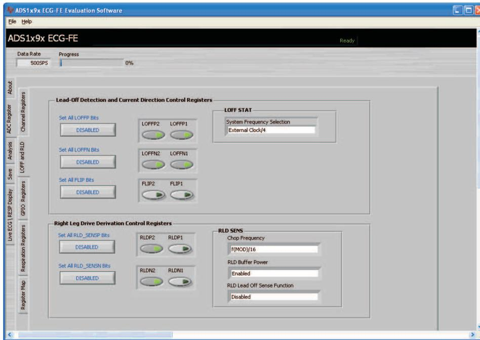
Figure 21. Register Configuration – LOFF and RLD
