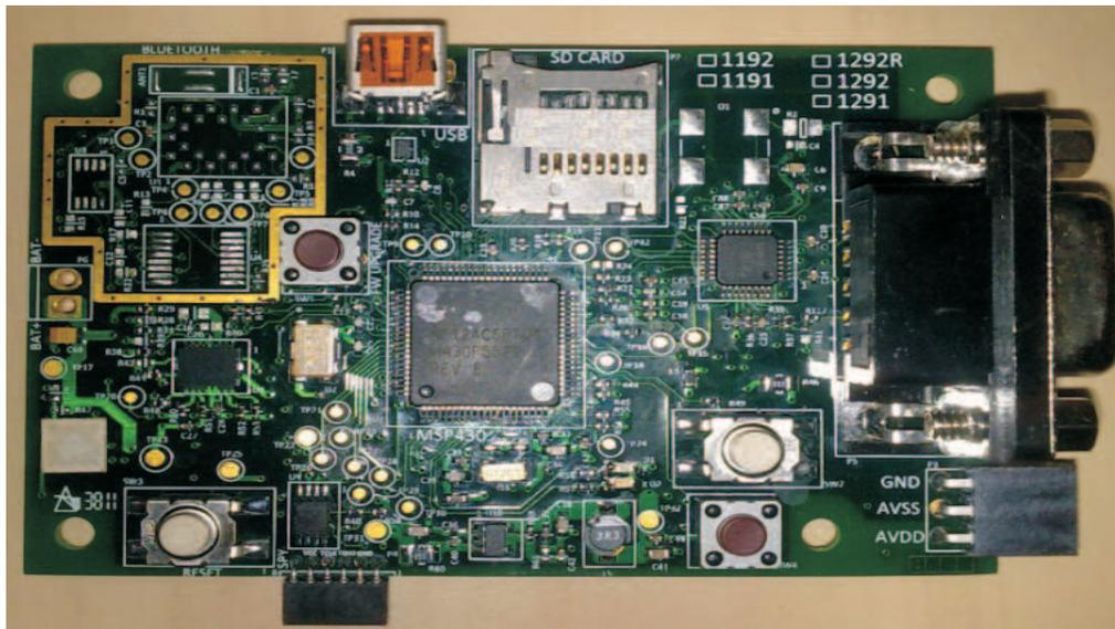
**Figure 1. ADS1x9xECG-FE Demonstration Kit**
