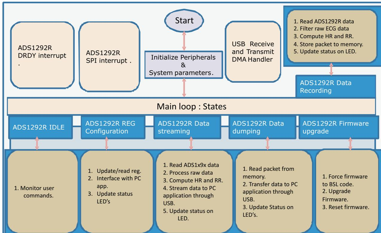
Figure 35. Firmware Architecture
