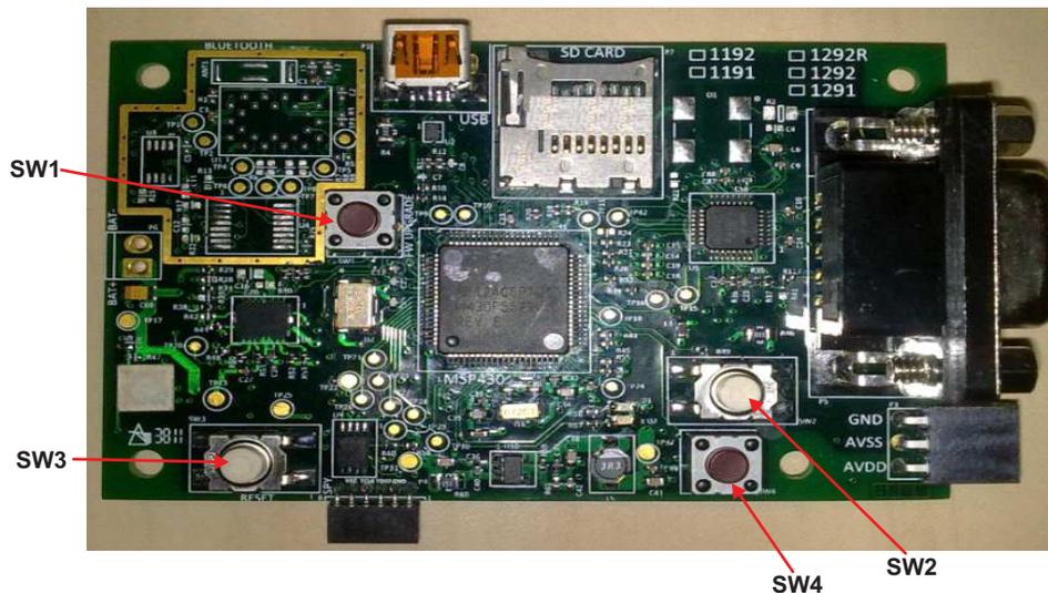
**Figure 34. Switch Positions**
