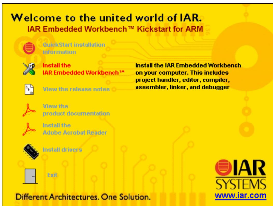
2. Click **Install the IAR Embedded Workbench** and follow the instructions in the installation application. If the files does not automatically open click open the file. We recommend that you use the default directories, and the **Full** installation option.
