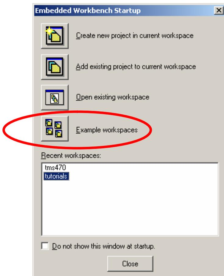
3. Navigate to the TexasInstruments\TMS470R1A256\ChipDemo example project. Check the “Do not prompt for working copy directory” box and click **Open**.
