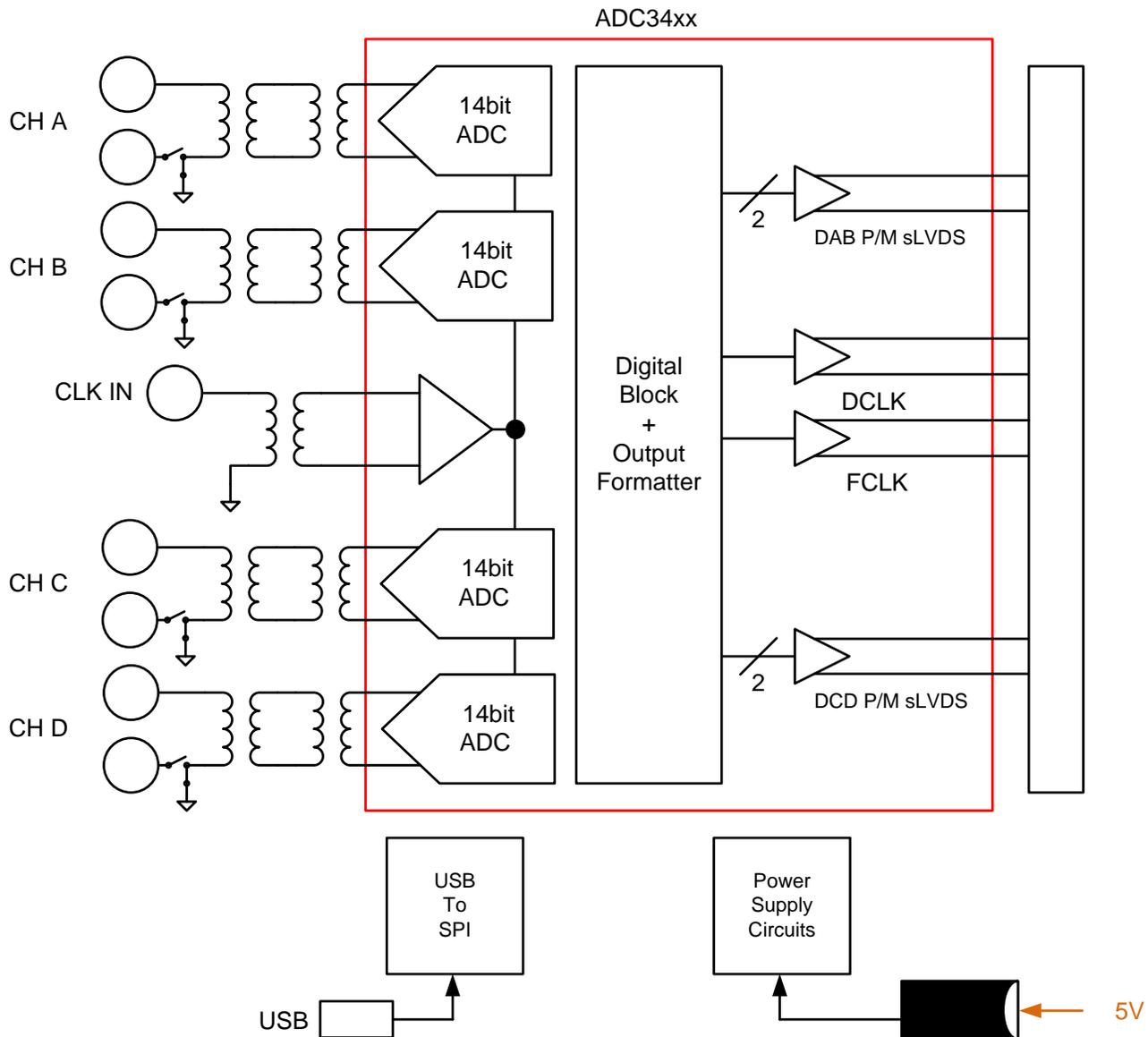
Figure 1. Simplified ADC344x EVM Block Diagram
