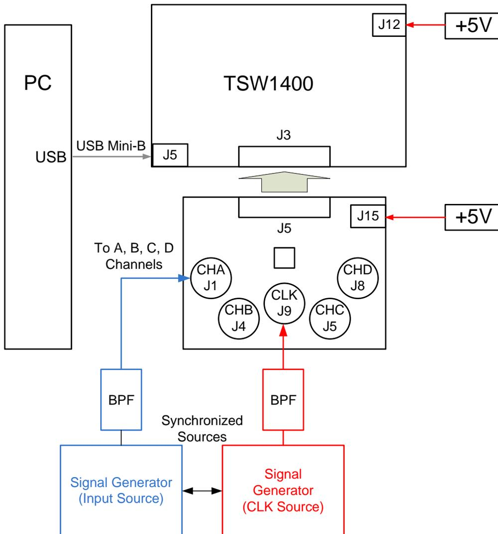
Figure 15. ADC32xx/ADC34xx and TSW1400 Test Setup Block Diagram
