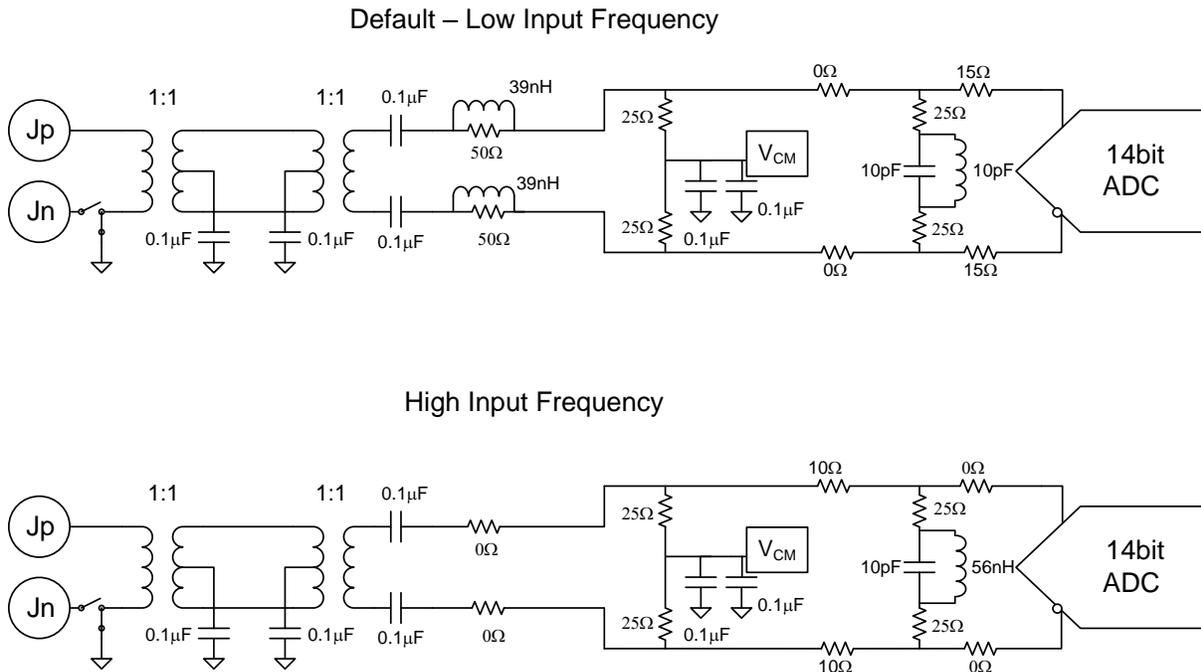
Figure 6. ADC3xxx ADC Input Circuit Options
