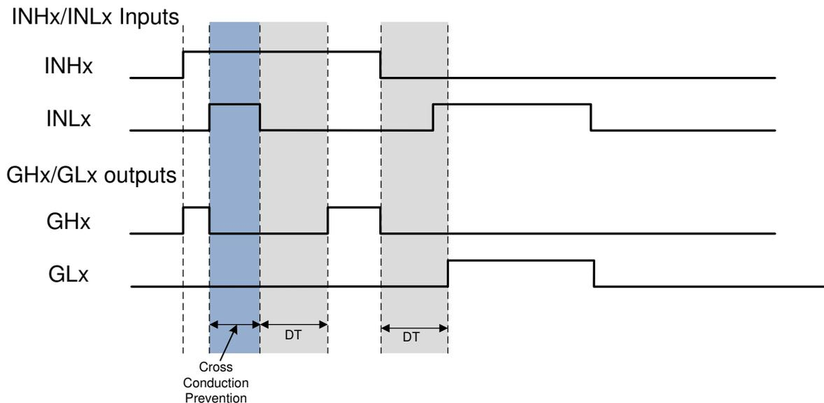
**Figure 8-2. Cross Conduction Prevention and Deadtime Insertion**
