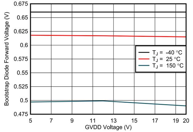
**Figure 7-6. Bootstrap Diode Forward Voltage over GVDD Voltage**
