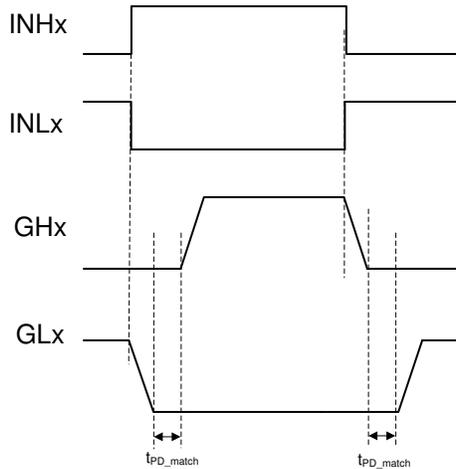
Figure 7-2. Propagation Delay Match (t<sub>PD\_match</sub>)
