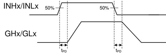
Figure 7-1. Propagation Delay (t<sub>PD</sub>)
