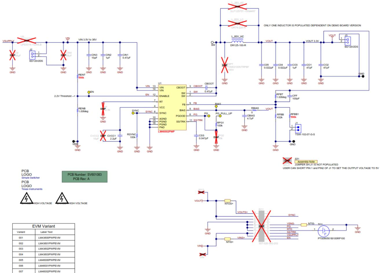
Figure 2. LM46002EVM Schematic
