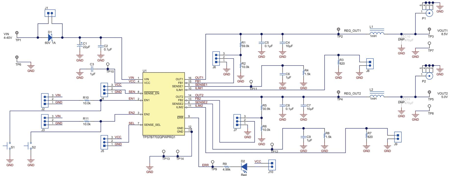
Figure 4. TPS7B7702EVM Schematic
