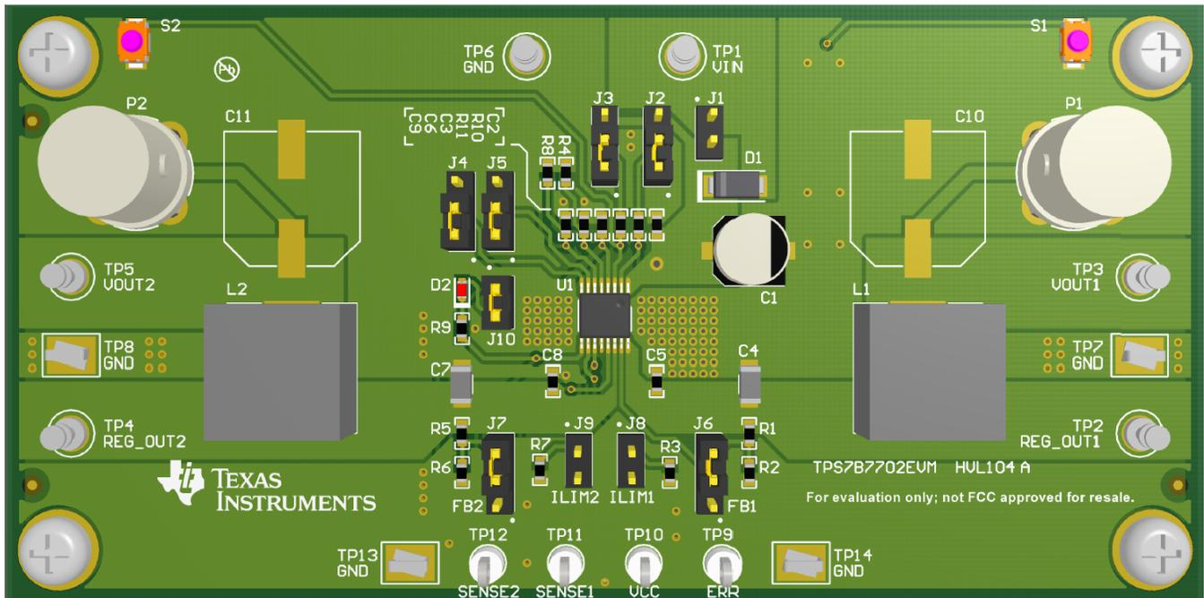
Figure 1. TPS7B7702EVM Component Placement (Assembly Top View)
