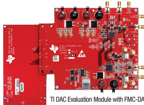
TI DAC Evaluation Module with FMC-DAC-Adapter Card Connection to Xilinx Evaluation Kit
