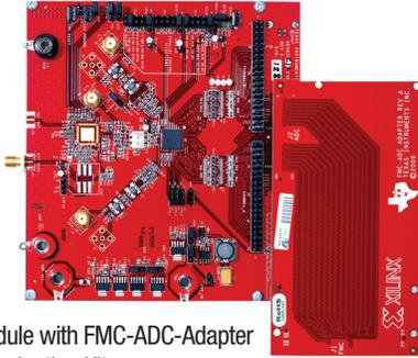
TI ADC Evaluation Module with FMC-ADC-Adapter Connection to Xilinx Evaluation Kit
