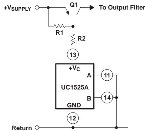
Figure 2. Grounded Driver Outputs For Single-Ended Supplies
