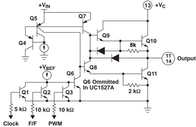
Figure 1. UC1525A Output Circuit (1/2 circuit shown)
