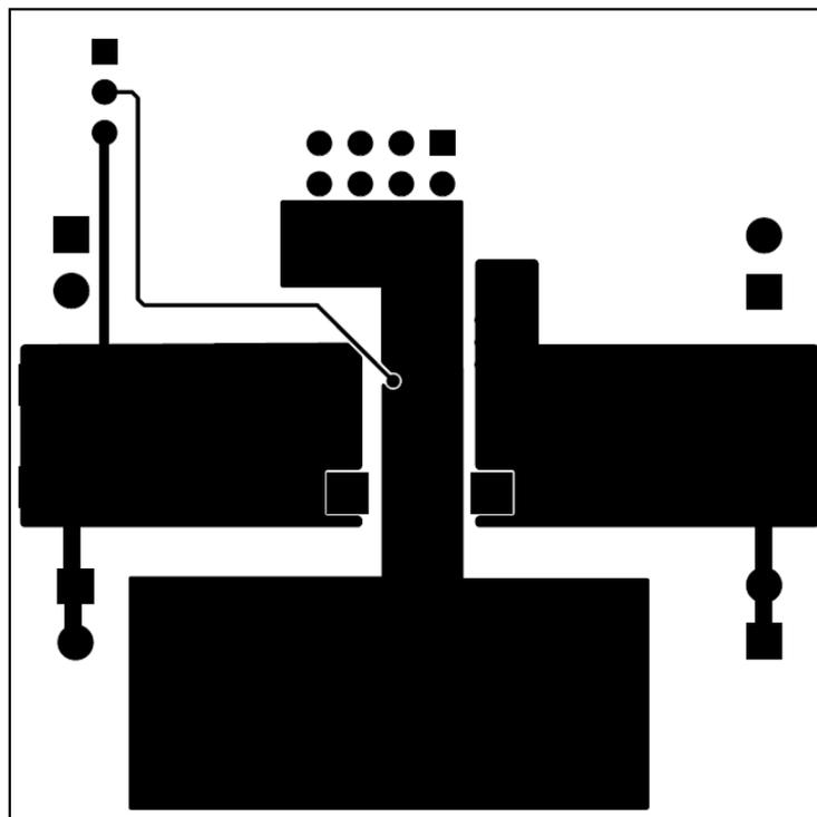
Figure 8. Bottom Layer Routing
