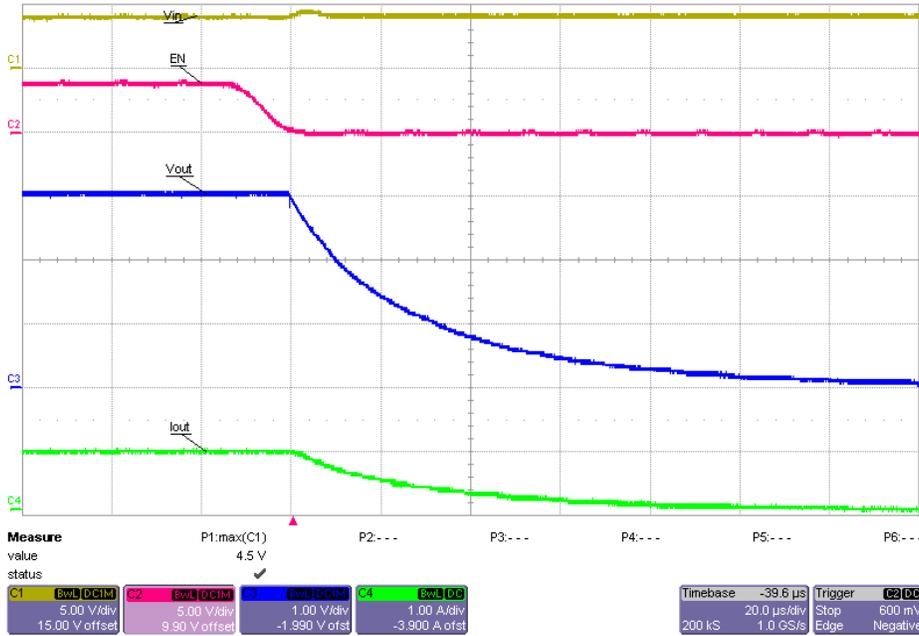
Figure 4. TPS7A8101 Shutdown with 3.3-Ω Load
