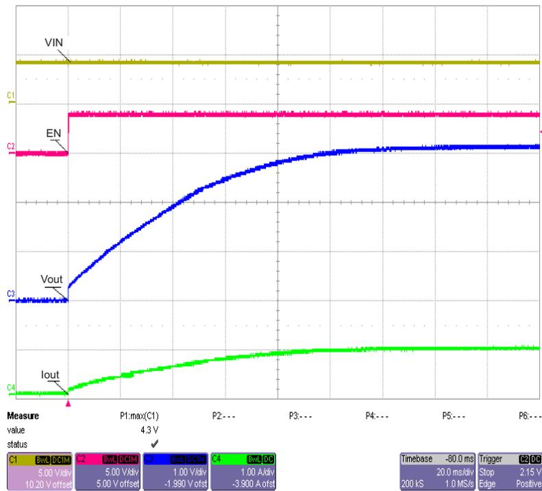
Figure 3. TPS7A8101 Start-Up Into Full Load, 1 A
