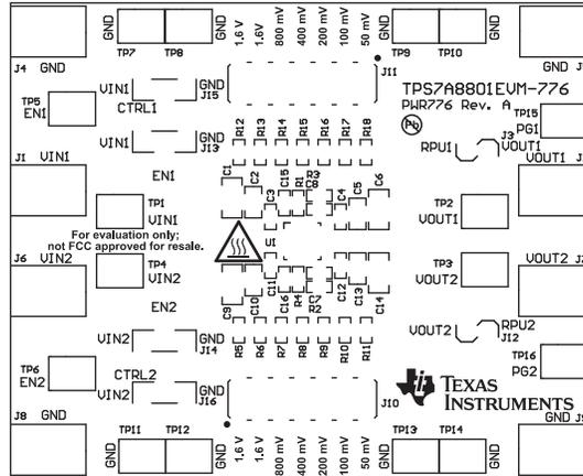
**Figure 1. Assembly Layer**
