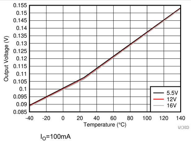
Figure 6-20. HO Low Output Voltage ( $V_{HoL}$ )
