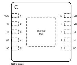
**Figure 5-4. DPR Package 10-Pin SON Top View**
