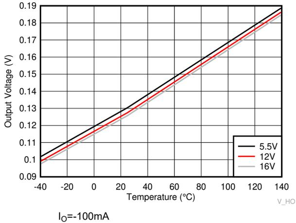
Figure 6-21. HO High Output Voltage ( $V_{HOH}$ )
