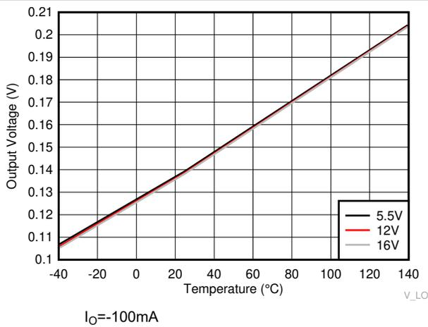
Figure 6-19. LO High Output Voltage ( $V_{LOH}$ )
