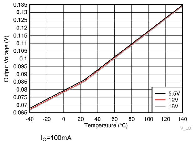
Figure 6-18. LO Low Output Voltage ( $V_{LOL}$ )
