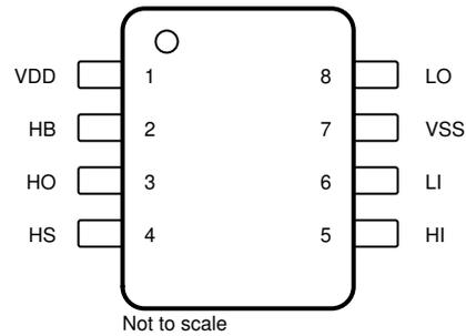
**Figure 5-2. D Package 8-Pin SOIC Top View**
