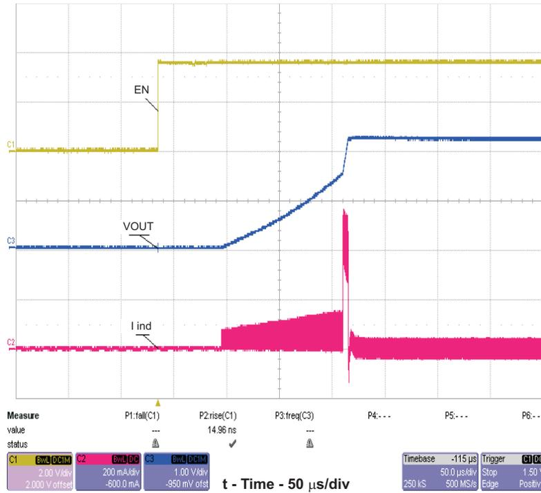
Figure 5. TPS62691 Start-Up Using EN With No Load, Vin = 3.6 V and Vout = 2.2 V
