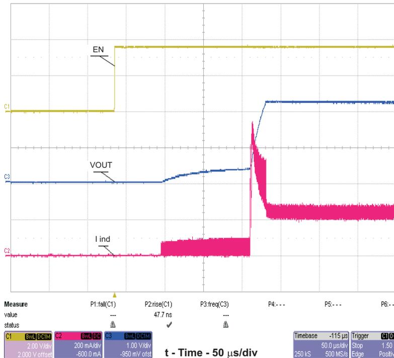
Figure 6. TPS62691 Start-up Using EN With 200-mA Load, Vin = 3.6 V and Vout = 2.2 V
