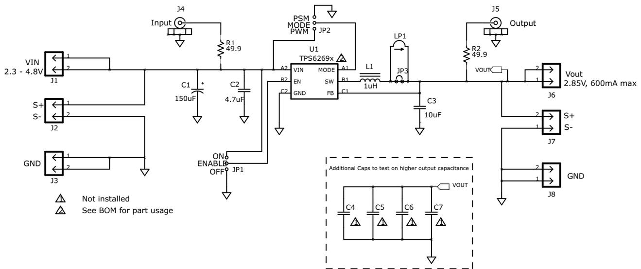
Figure 1. TPS6269xEVM Schematic
