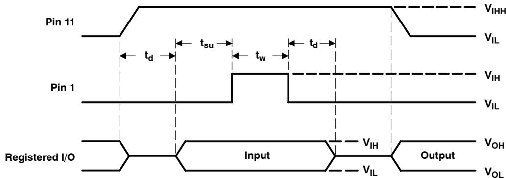
NOTE 3:  $t_d = t_{su} = t_h = 100$  ns to 1000 ns  $V_{IHH} = 10.25$  V to 10.75 V
