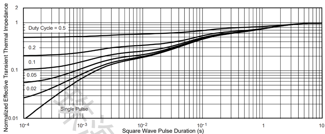
Fig 13. Normalized Thermal Transient Impedance, Junction-to-Foot
