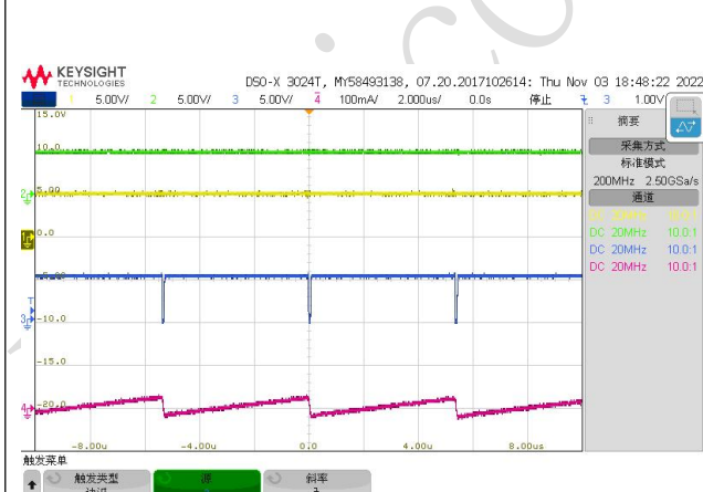
CH1:EN CH2:Vout CH3:SW CH4:IL Vin=24V Vout=5V Fig.14 Start up waveform through EN, Iout =0A
