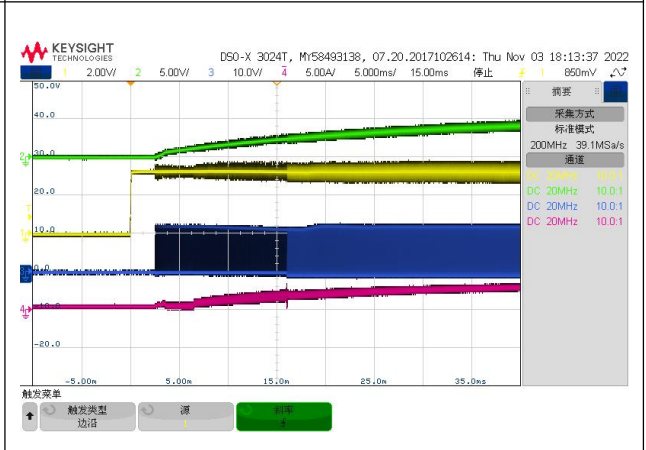
CH1:EN CH2:Vout CH3:SW CH4:IL Vin=12V Vout=5V Fig.11 Start up waveform through EN, Iout =3A
