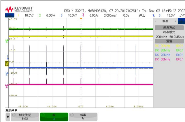
CH1:Vin CH2:Vout CH3:SW CH4:IL Vin=24V Vout=5V Fig.20 Steady State waveform Iout =0A
