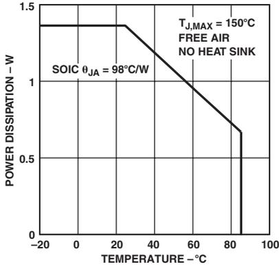
TPC 28. Maximum Power Dissipation vs. Ambient Temperature
