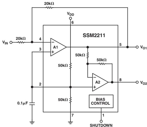
Figure 1. Simplified Schematic
