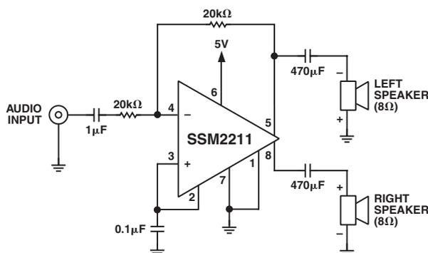
Figure 9. SSM2211 Used as a Dual Speaker Amplifier
