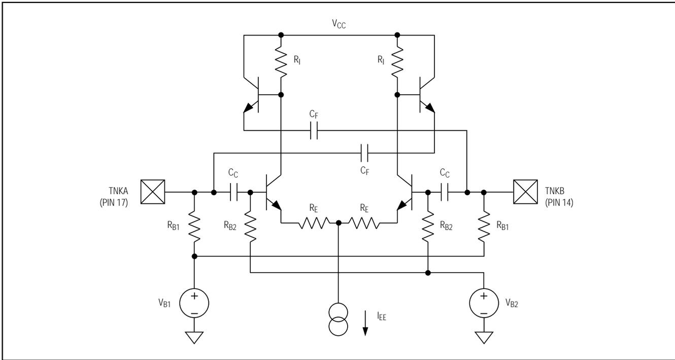
Figure 15. Simplified Input Network for VCO Resonator Ports
