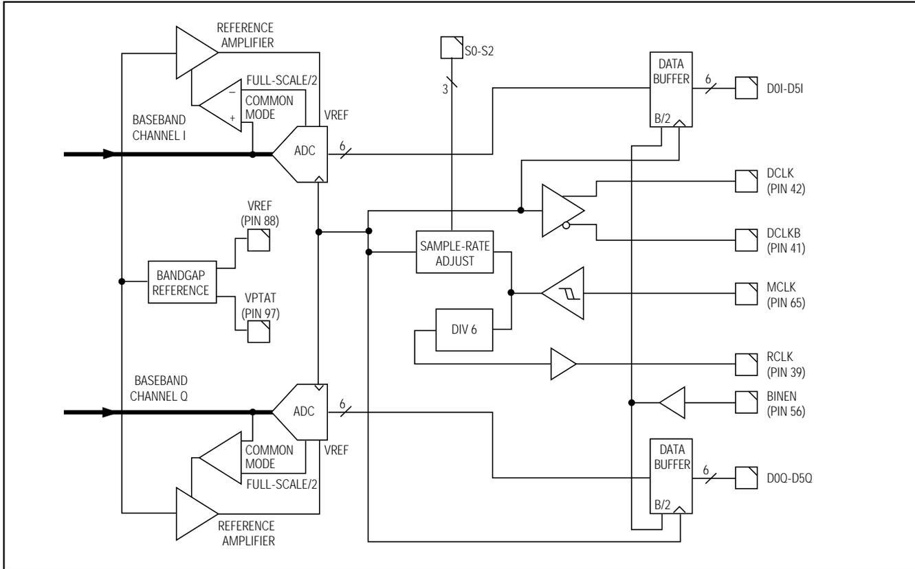
Figure 4. Functional Diagram—MAX2101 ADCs and Supporting Sections
