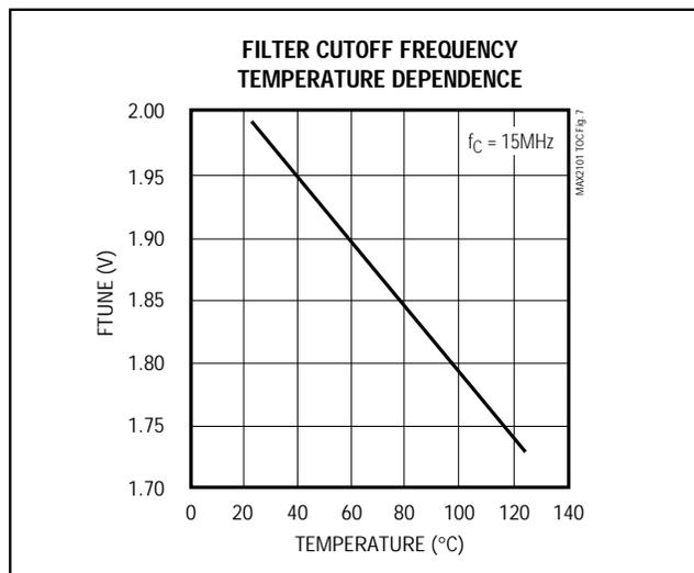
Figure 7. Typical Filter Cutoff Frequency Temperature Dependence
