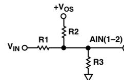
Figure 6. Scaling and Offsetting AIN(1-2) for Bipolar Inputs
