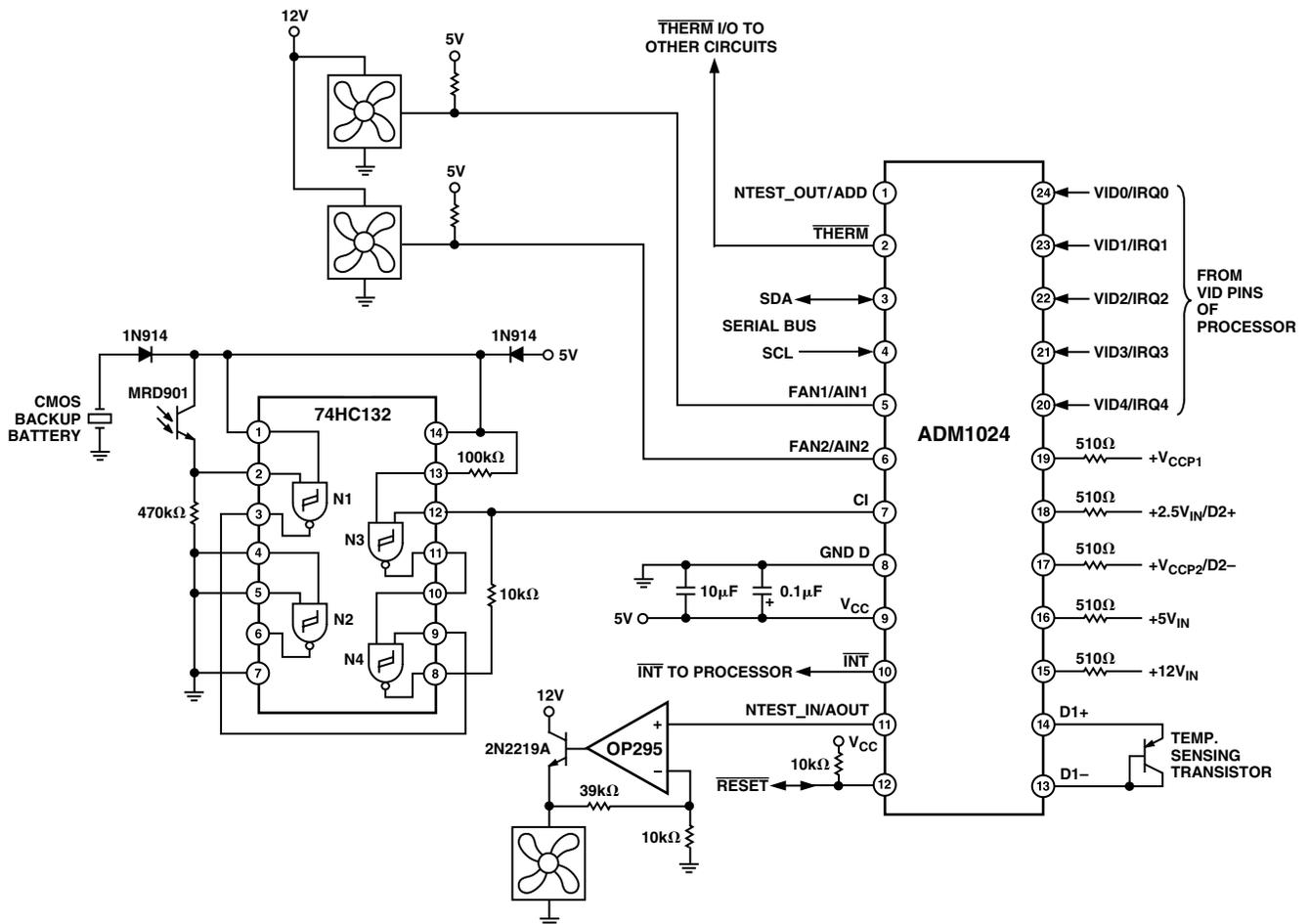
Figure 18. Application Circuit
