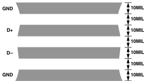
Figure 8. Arrangement of Signal Tracks
