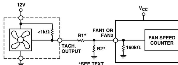
Figure 10d. Fan with Strong Tach. Pull-Up to >V<sub>CC</sub> or Totem-Pole Output, Attenuated with R1/R2
