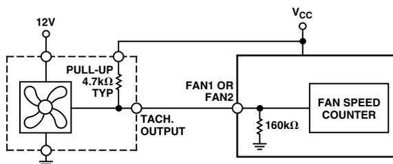
Figure 10a. Fan with Tach. Pull-Up to +V<sub>CC</sub>
