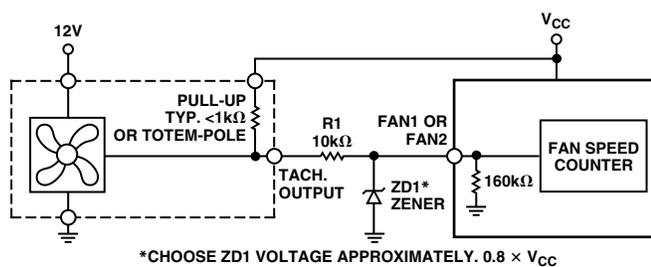
Figure 10c. Fan with Strong Tach. Pull-Up to >V<sub>CC</sub> or Totem-Pole Output, Clamped with Zener and Resistor
