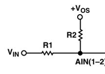
Figure 5. Scaling and Offsetting AIN(1-2) for Negative Inputs
