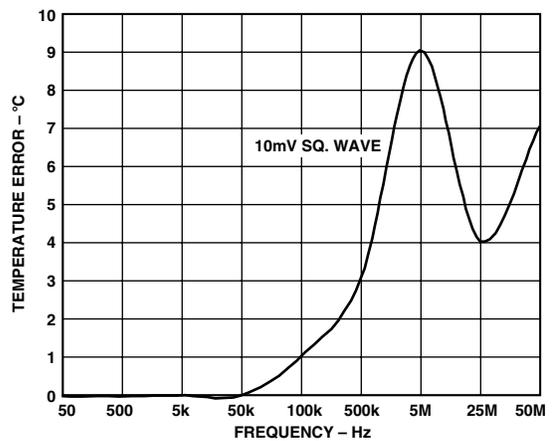
TPC 6. Temperature Error vs. Differential-Mode Noise Frequency
