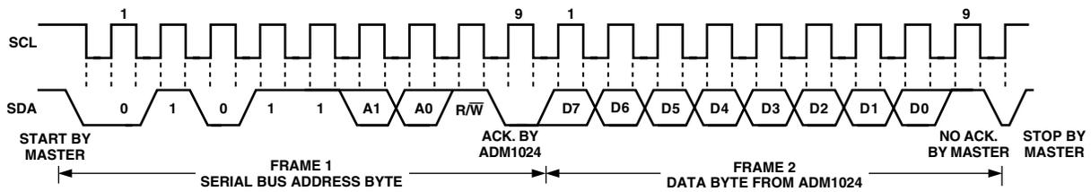
Figure 2c. Reading Data from a Previously Selected Register
