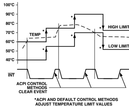
Figure 15. Operation of  $\overline{\text{INT}}$  for Temperature Interrupts
