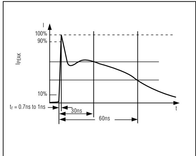
Figure 9. IEC 1000-4-2 ESD Generator Current Waveform
