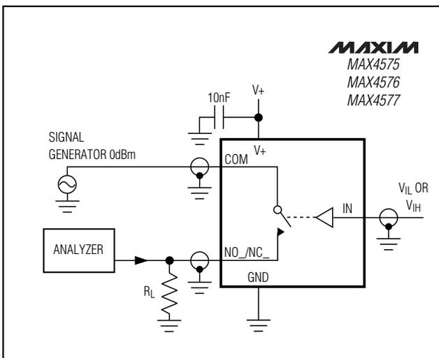
Figure 2. Off-Isolation/On-Channel Bandwidth
