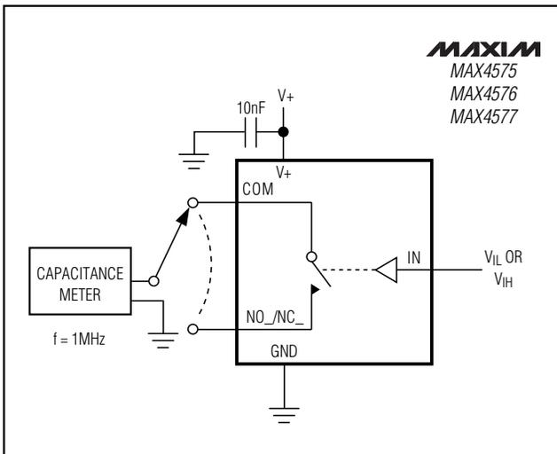
Figure 4. Channel Off/On-Capacitance
