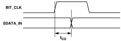
Figure 6. Propagation Delay
