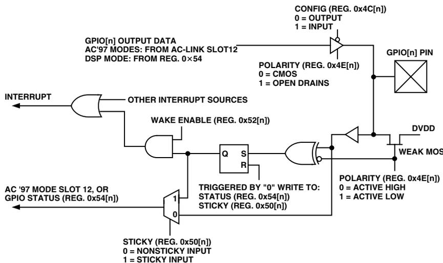
Figure 11. Conceptual Diagram of GPIO Pin Behavior
