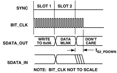
Figure 7. AC Link Low Power Mode Timing
