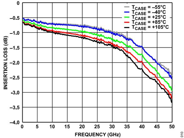
Figure 9. Insertion Loss vs. Frequency Without Impedance Match
