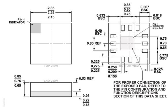
**Figure 26. 12-Terminal Land Grid Array [LGA]
