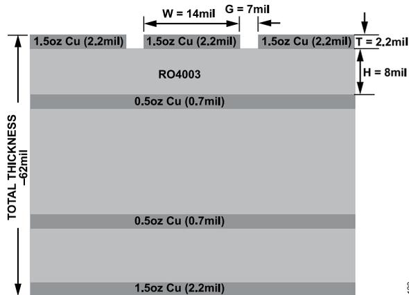
Figure 22. Probe Matrix Board (Cross Section View)
