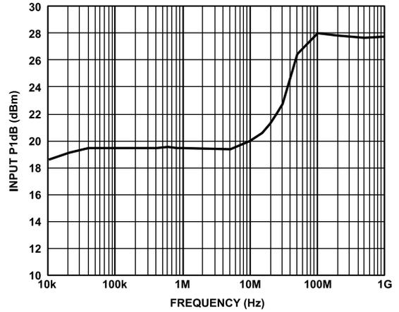
Figure 15. Input P1dB vs. Frequency (Low Frequency Detail)
