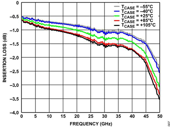
Figure 7. Insertion Loss vs. Frequency with Impedance Match
